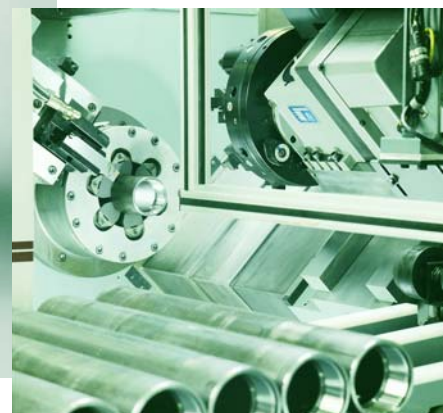
1.00" to 5.500" with special collet that covers plus/minus 0.375" variation in material OD size with quick change collet pads.
