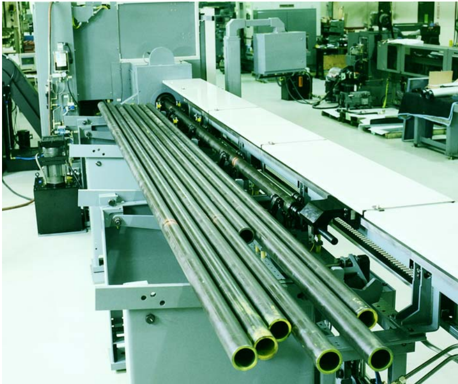
Automatic magazine tube and bar loader is available to feed stock from 6 to 60 feet.
