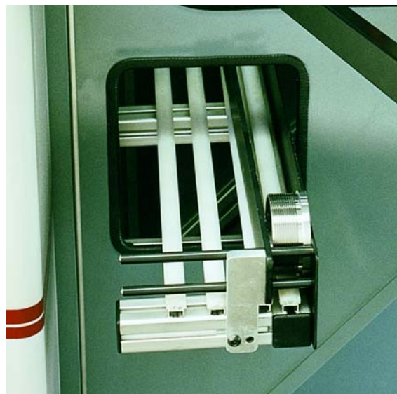
Automatic stripper attachment with part delivery chute.
