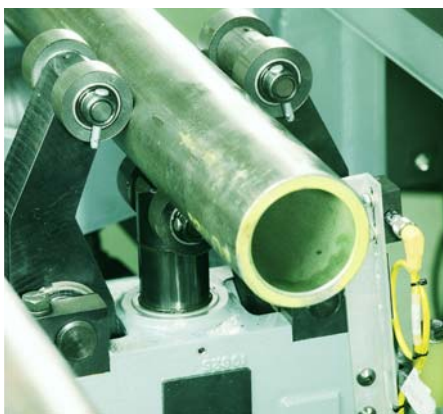
Long tubes and bars are supported with the loading table steady rest system. No adjustment is required for different stock diameters.
