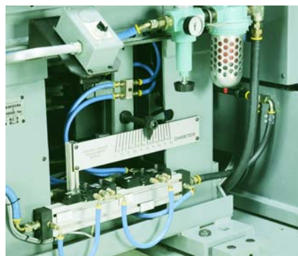
Stock diameter changeover is fast and easy with our electric screw-driven height adjustment.
