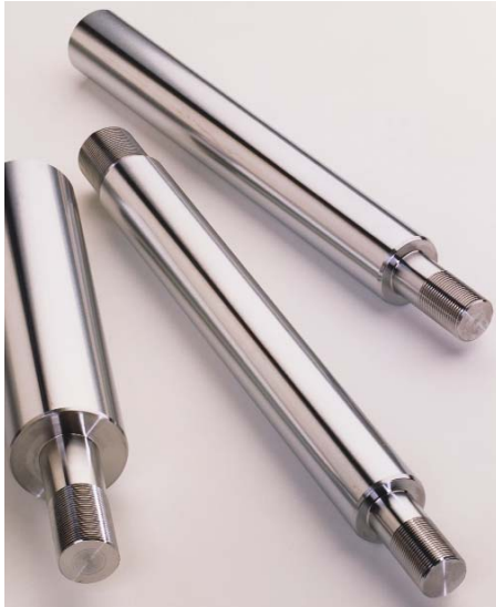
Piston rods to 3.5" (88.9-mm) OD are machined complete from chrome-plated bar on the Bardons & Oliver ISC 350 CNC lathe.
