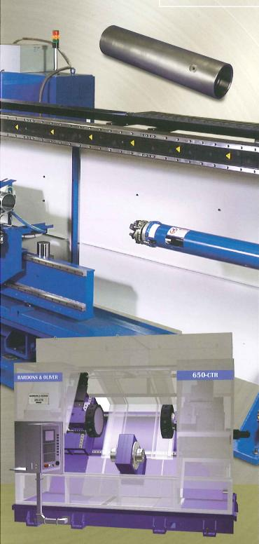
The third machine in this family of high-efficiency turning machines is the center drive lathe. Parts are gripped in the middle while complex machining is performed on both ends at the same time. No re-gripping or relocating of the part allows the highest specifications to be met. The result is dead true tolerances, held end-to-end, unmatched by any other configuration of turning center.
